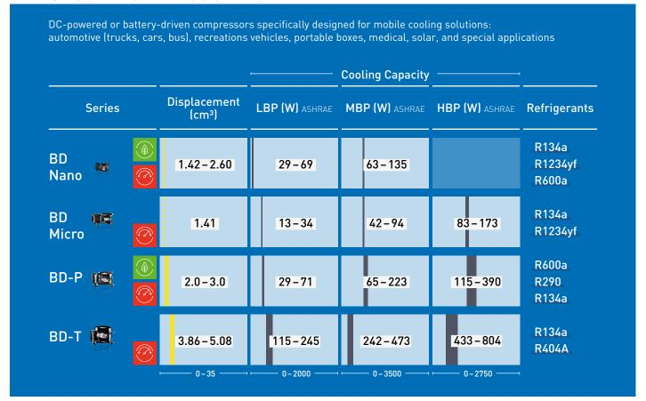
Secop mobile cooling compressors are available for a variety of DC voltage ranges and certain controllers even feature an AC option for various mains supply.
