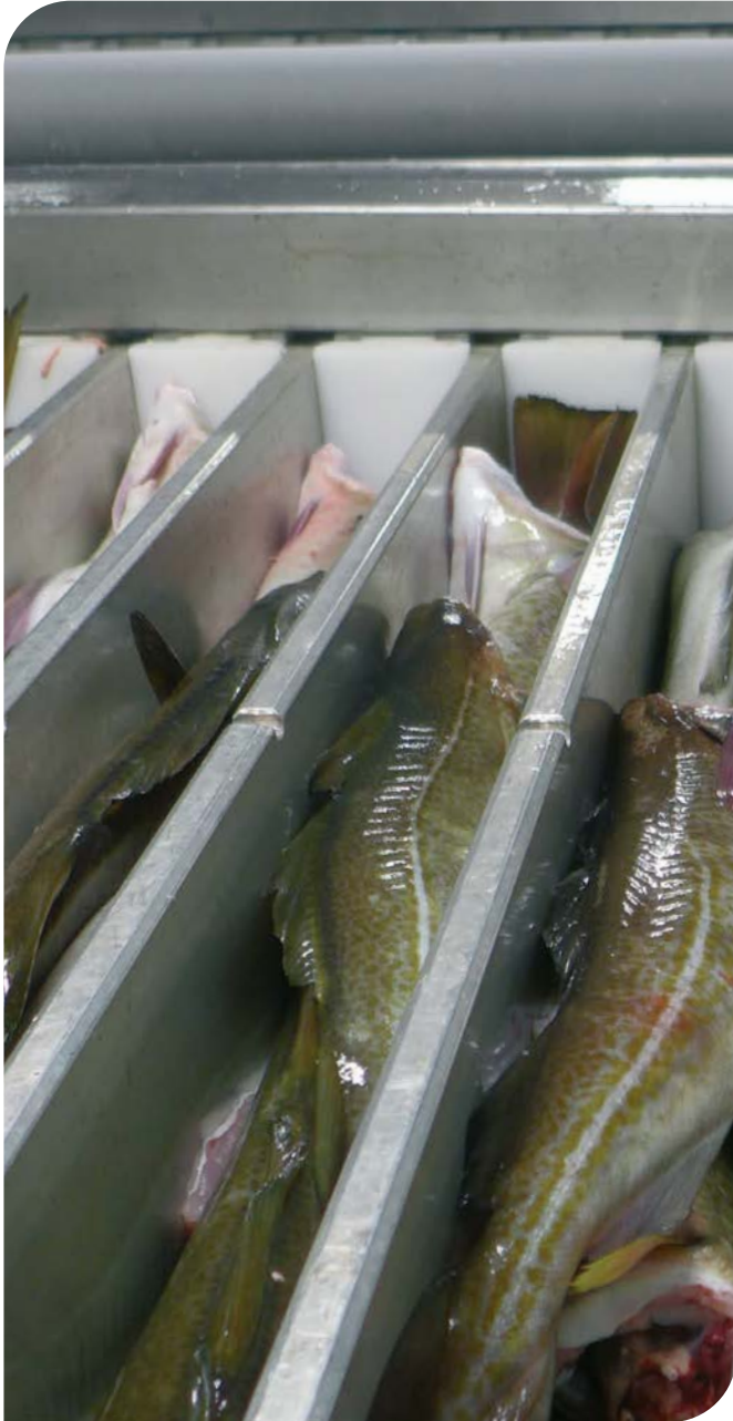
Figure 5 | Cod frozen in vertical plate freezers. (photo: Guro M. Tveit, SINTEF Ocean)
